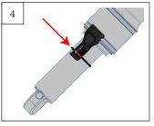
WARNING: Make sure the sag indicator does not contact the frame or linkage through the suspension cycle. Otherwise, the indicator may break while riding.
