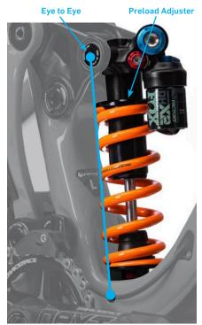
Spec rates should match the average rider for the frame size but some riders may need a lighter or heaver spring to achieve the recommended 30% sag. Listed below are the recommended spring rates based on rider weight as well as coil length and spring stroke specifications for the spring required to run on FOX and Marzocchi coil-over shocks used on the Mach 6.
